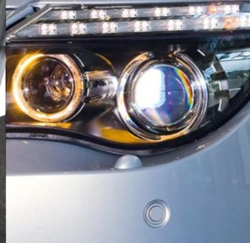
**ULTRASOUND CAN BE USED TO PUNCH VARIOUS GEOMETRIC SLOTS AND WELD ON PARKING SENSOR MOUNTS**
