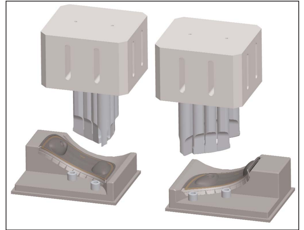
The application is carried out in two process steps with mirrored tools.
