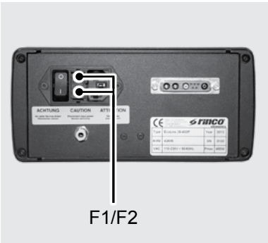
Fig. 53: Generator fuses in the installation area
