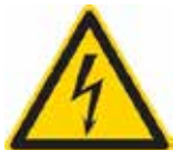
Beware of dangerous electrical voltage
